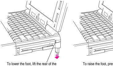
I o lower the foot, lift the rear of the computer and press the release button. The foot extends automatically.
